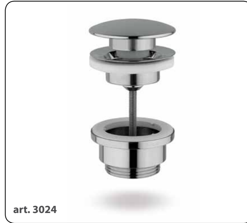
Vidage 1"1/4, "UNIVERSALE" lavabo, tappo ottone Ø72mm, système de commande toujours ouvert Pop-up waste 1"1/4, washbasin "UNIVERSAL" model, brass plug Ø72mm, "always open" control system
