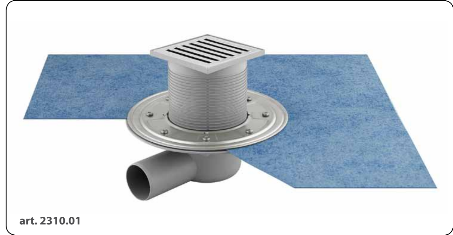
Kit siphon d'évacuation + gaine d'étanchéité pré-formée. Grille 105x105 mm, épaisseur 5mm, mod. "LINEA" Siphon drain kit. Completely removable. Comes with pre-sized isolation membrane. Design grid 105x105 mm, thickness 5 mm, "Linea" model. Side outlet Ø 50 mm. Height 79 mm.
